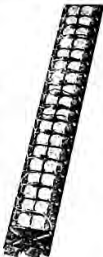
Fig. 3. Cylindrical electrostatic loudspeaker. Each strip carries the full frequency range and the sections are coupled to form an electrical transmission line. The inductor assembly is shown below.
